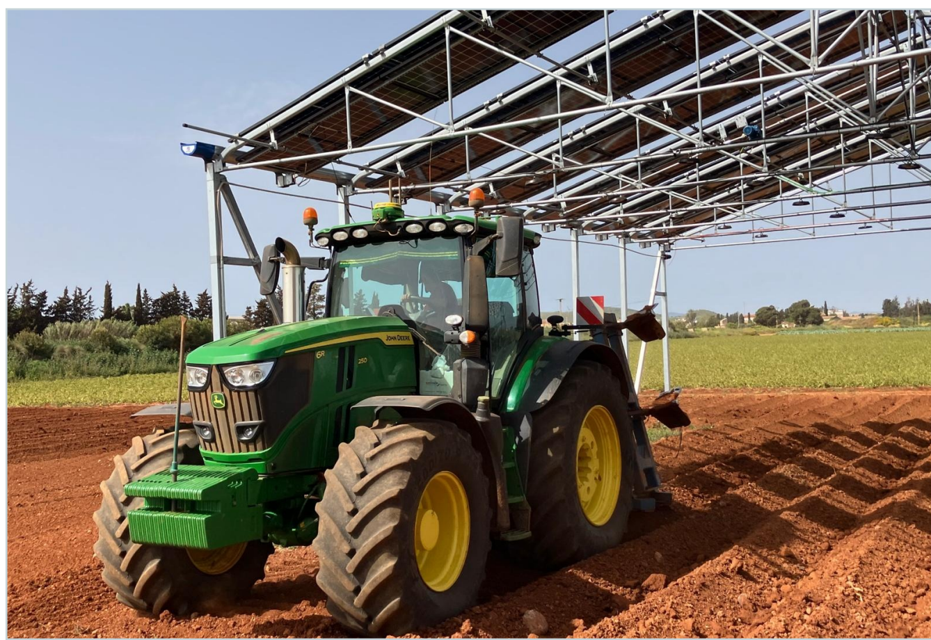
Fig. 2. VOLTAGRO prototype at El Algar: a conventional tractor with a mounted plough working under the elevated canopy.
